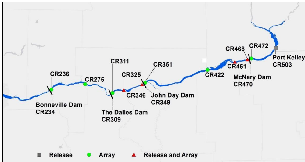
Figure 41. Map Showing Sites of Fish Releases, Dam-Face Arrays, and Autonomous Node Arrays for Summer 2014. Fish will be released from the most upstream location in the study at Port Kelley but will not have an autonomous node array (grey box), four fish release sites having autonomous nodes (red triangles), six arrays of autonomous nodes (green circles) and two double arrays of cabled hydrophones at McNary and John Day Dams. Columbia River (CR) km upstream of the river mouth and the Pacific Ocean is listed after each site label.
