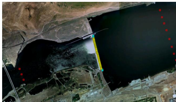
Figure 12. Satellite Image of McNary Dam (MCN) (Courtesy of Google Earth) Showing Locations of Underwater Acoustic Receivers. Yellow icons show locations of slotted pipes on every pier adjacent to spill bays and turbines. Exact elevations of deployed hydrophones will be determined after a thorough evaluation of the acoustic environment in the forebay. Each pipe will receive two trolleys for deploying one deep and one shallow hydrophone at each pier. Blue icons at the ends of the dam indicate locations of single hydrophone deployments to detect fish approaching from the north or south shores. Also shown as red squares are eight autonomous nodes in a forebay entrance array located about 2 km upstream from the dam (right side) and three autonomous nodes in a tailrace egress array located about 2 km downstream of the dam.
