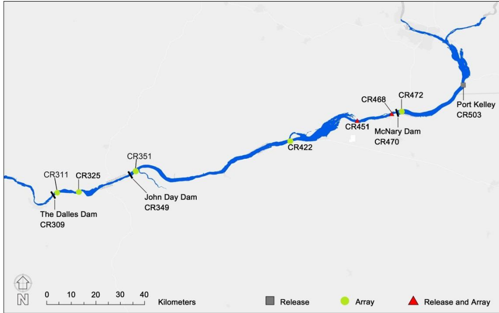
Figure 30. Map Showing Sites of Fish Releases, Dam-Face Arrays, and Autonomous Node Arrays for Spring 2014. Fish will be released from most upstream location in the study at Port Kelley but will not have an autonomous node array (grey box), two fish release sites having autonomous node arrays (red triangles), five sites will have only arrays of autonomous nodes (green circles) and a double array of cabled hydrophones will be deployed at McNary Dam. Columbia River (CR) km upstream of the river mouth and the Pacific Ocean is listed after each site label.
